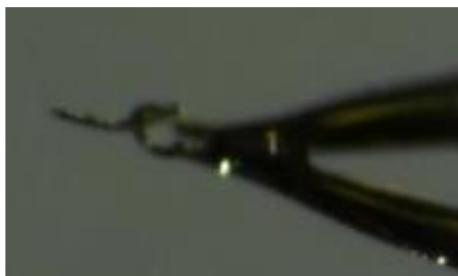
Figure S24 Bent crystal used for data collection.
