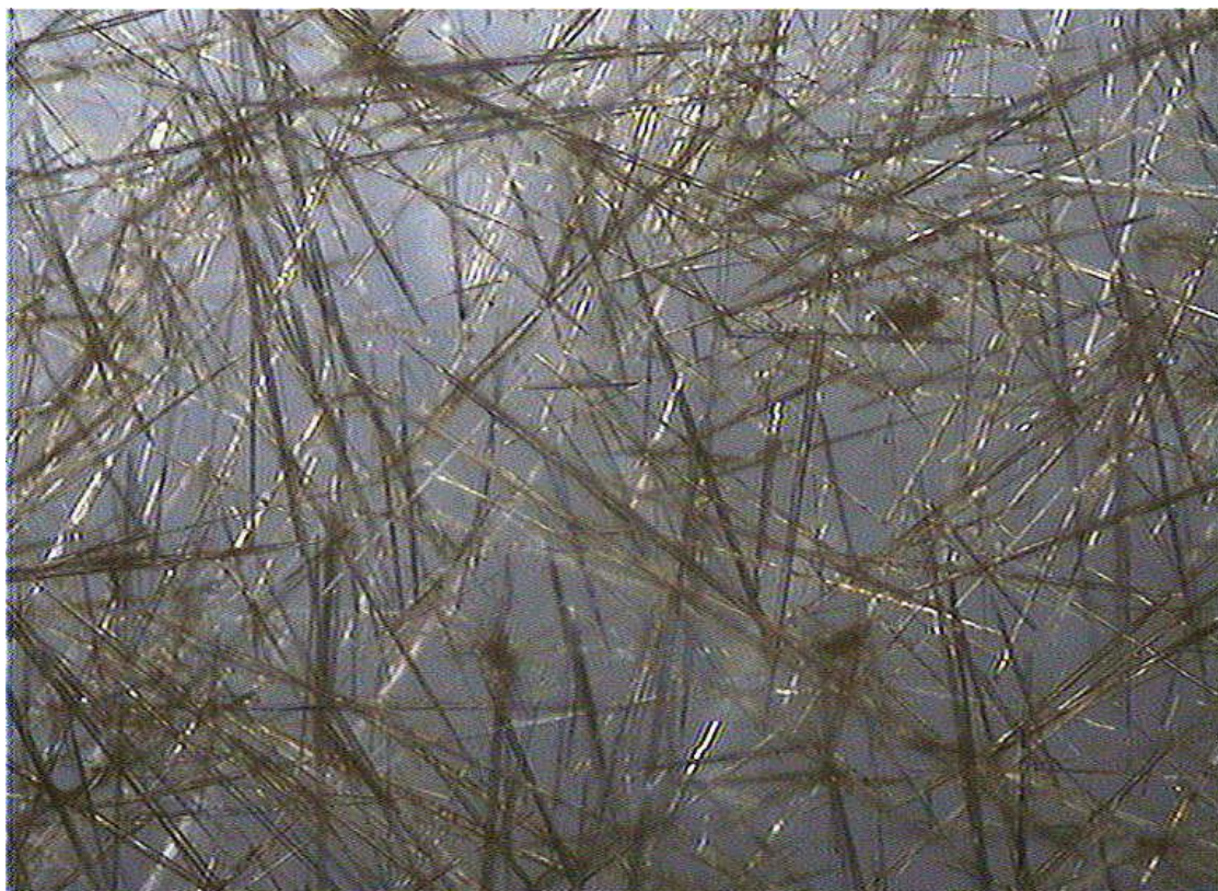
Figure S1 A typical photographs of crystals of 1 taken under microscope. All the solvent combinations and conditions used to get the curved crystals of 2 has been tried for 1 . But all these conditions yielded only long rods as shown in Figure S1. No curved crystals were observed in the bulk.
