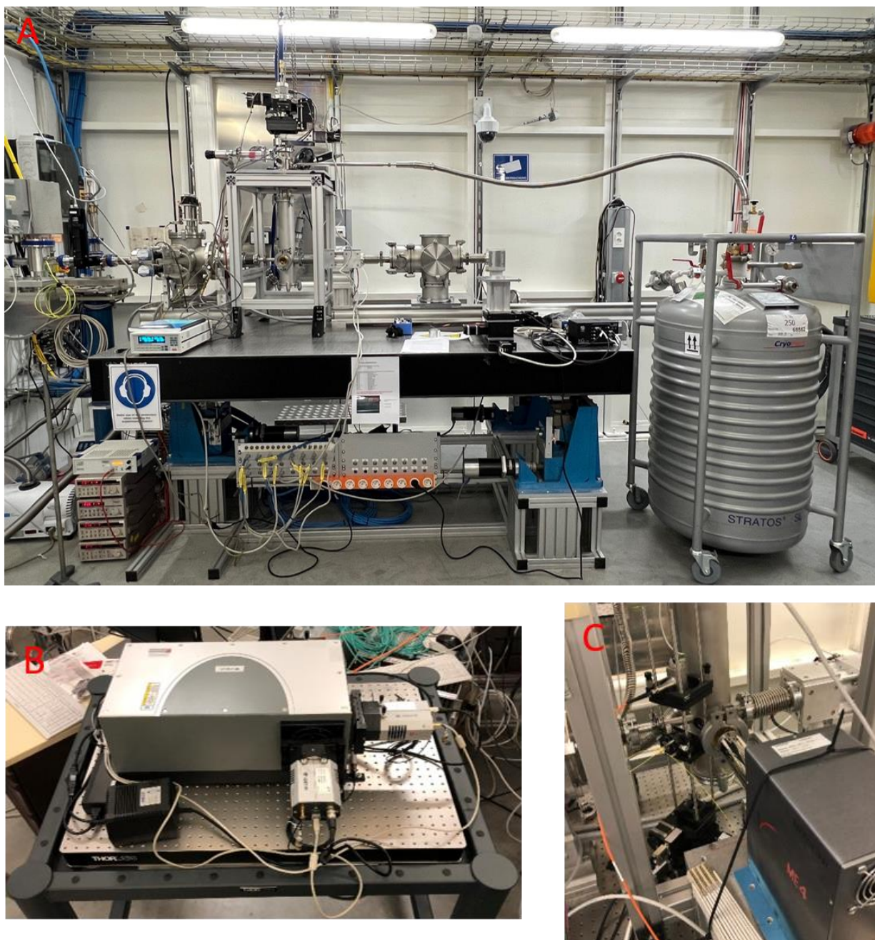
Figure S1 (A) Photograph showing the He –flow cryostat and vacuum chamber integrated into the end station of the P65 beamline. (B) Photograph showing the optical spectrometer and detectors. (C) Photograph showing the optical head aligned in front of the optical viewport.
