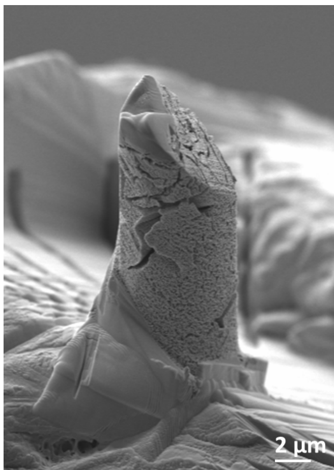
Figure S2 Scanning electron micrograph of a nanoporous gold sample pillar after to lift-out and transfer.
