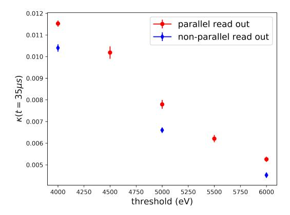
Fig. 3. Dependence of the correction parameter  $\kappa$  on the set threshold value and read out mode.
