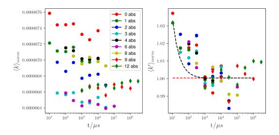
Fig. 2. a) Mean number of photons registered per pixel, normalized on the incoming flux, exposure time and absorber transmission. b) Data also normalized on  $\langle k_{norm} \rangle$  for exposure times of t=1 ms  $\leq t \leq 10$  ms.
