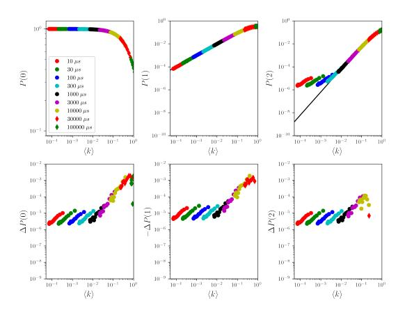
Fig. 1. Top row: Distribution of photon count probabilities as a function of number of photons per pixel  $\langle k \rangle$ , measured with the PSI Eiger 500k at beamline ID02, ESRF. In black, the expected Poisson-Gamma distribution is plotted. Bottom row: Difference between expected and measured photon count probabilities for k=0,1 and 2 photons.
