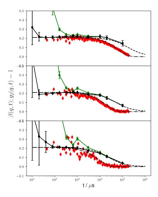
Fig. 4. XPCS and XSVS measurements on 100 nm silica particles at q-values of 1.75  $10^{-2}$  nm<sup>-1</sup>, 3.25  $10^{-2}$  nm<sup>-1</sup>, and 4.75  $10^{-2}$  nm<sup>-1</sup>. The green data points correspond to the uncorrected and the black data points to the corrected XSVS results.
