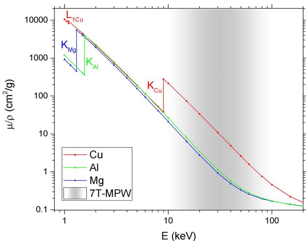
**Figure S1** X-ray mass attenuation coefficients of Cu, Al and Mg from 0.8 to 200 keV.
