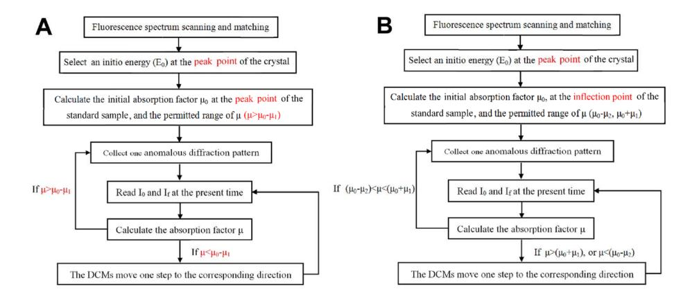
**Figure S1** Flow chart of peak-peak monitoring (A) and inflection-peak monitoring (B) of the incident X-ray energy. The steps that are different from the inflection-inflection monitoring are colored in red.
