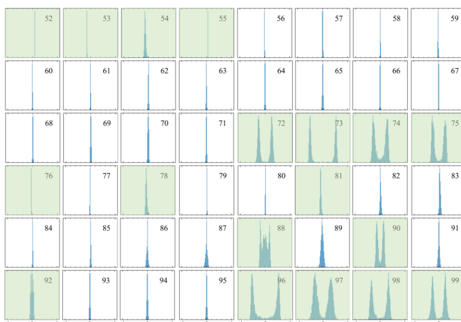
Figure S3. Multi-convergence mode-amplitude histograms for each of the displacive-mode amplitudes for the O1 and O2 oxygen sites in BNN. The displacive modes highlighted in green was selected to the initial mode set. The horizontal axis of each plot goes from -1 to 1 Å, with tick marks every 0.2 Å. With respect to the polar P4bm structure of BNN, modes 52-75 acts on O1/d, modes 76-99 on O2/d.
