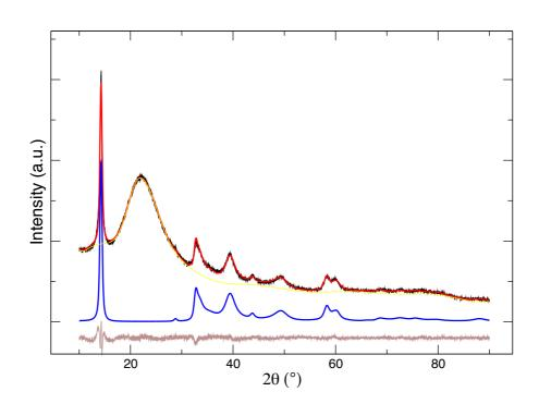
**Figure S1** Fitting of the prismatic-octahedral model to the XRD data of the exfoliated-restacked MoS<sub>2</sub> sample. Experimental, black; calculated, red; background, yellow; model, blue; residual, brown.
