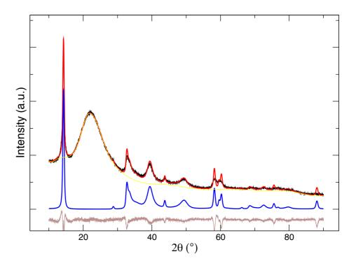
**Figure S2** Simulation of the prismatic-octahedral model to the XRD data of the exfoliated-restacked MoS<sub>2</sub> sample. Experimental, black; calculated, red; background, yellow; model, blue; residual, brown. The correlated interatomic distance uncertainty is eliminated.
