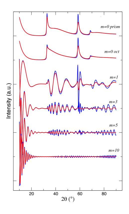
**Figure S3** Components of the total XRD pattern corresponding to different height jumps (see text) between S-Mo-S sandwiches. Blue traces, no interatomic distance correlated uncertainty; red traces, with correlated uncertainty. For m=0 (self-scattering of the S-Mo-S units) the distinct contributions of prismatic and octahedral sandwiches are drawn.
