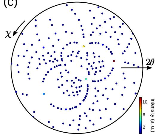
Fig. S1. Laue diffraction of single-crystal KCl of the B1 structure. (a) Example code. (b) 2D diffraction pattern on a planar detector. Pink star: direct beam. (c) Corresponding  $\chi - 2\theta$  plot in the polar coordinate system.
