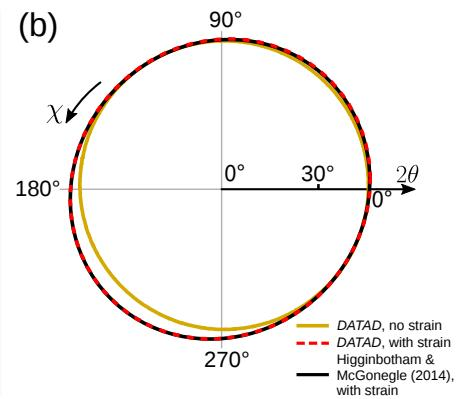
Fig. S2. (a) [Example code](#) that simulate the diffraction rings of strained Fe specimens. (b)  $\chi - 2\theta$  plots in the polar coordinate system for strain-free and strained Fe specimens obtained from *DATAD* and Higginbotham & McGonegle (2014).
