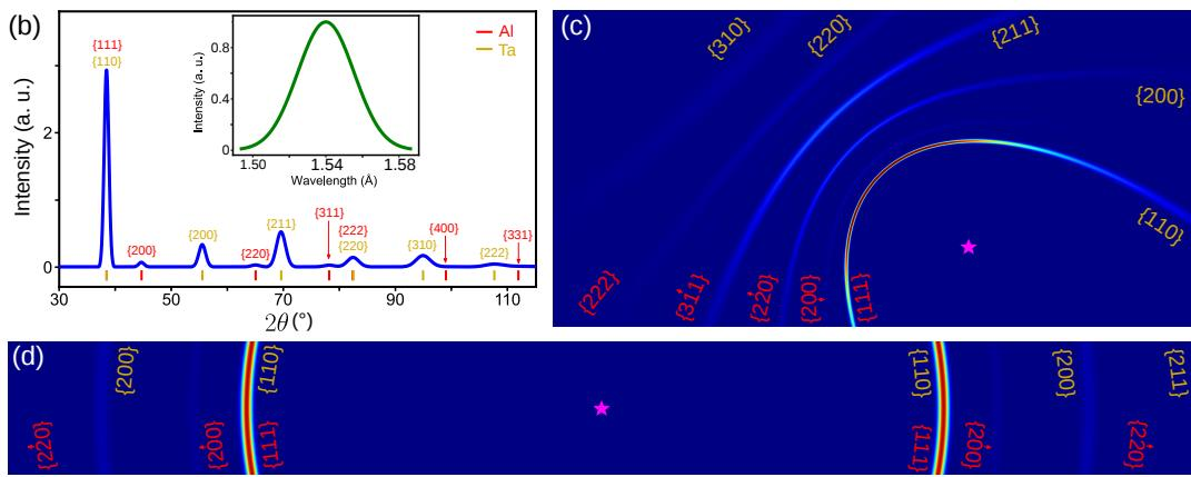
Fig. S3. Bragg diffraction of a mixture of ideal polycrystalline Ta and Al. (a) [Example code](#). (b) 1D diffraction curve. Inset: X-ray spectrum. (c) 2D diffraction pattern projected on a planar detector. (d) 2D diffraction pattern projected on a cylindrical detector (expanded).
