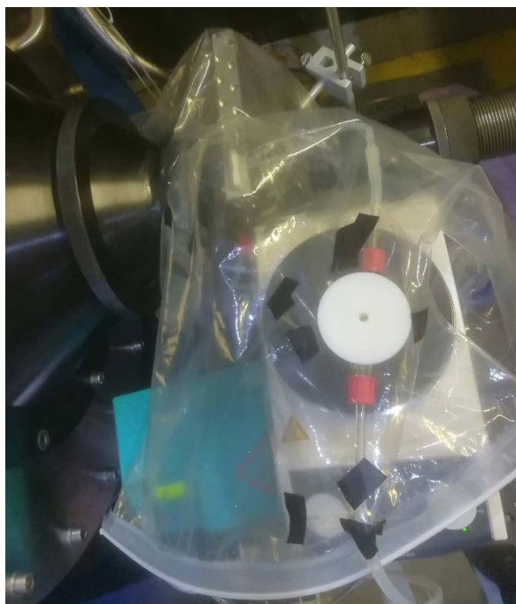
Figure S2 Photograph of the free-film setup at beamline D11 with the Helium bag (top-view)
