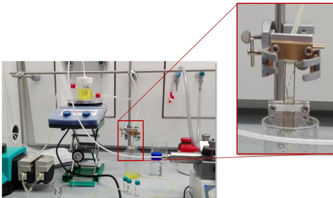
Figure S1 Photograph of the free-film setup in the laboratory, pumping an aqueous CdS nanoparticle suspension for better visibility of the free-film between the wires in the enlarged area.
