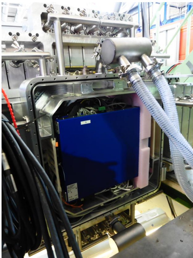
Figure S2 View of the detector from the rear: the air box (open in this photo, the cover is removed), the internal switches (Hirschmann) and the exhaust airline with the power and signal cables through the hoses can be seen. The photo was taken during the assembling phase of the new detector on KWS-2.
