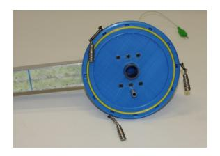
Push M4 hex nuts into slots on Dewar lid and use M4x20 screws to attach arbitrary fasteners. These serve to lock the lid to the Dewar. The image shows a simple system of springs and hooks, which can slide into catches supported by a metal strip around the Dewar body.
