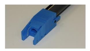
Thread thermistor wire through the coldhead, leaving some slack. Push-fit the thermistor guide tube into coldhead opening.
