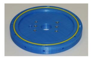
Repeat on underside. Press M4 hex nuts into nutcatches.
