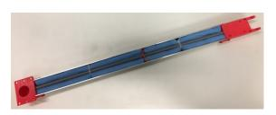
Place tubing assembly into U profile and use cable ties to fix foam sheets to tubes. Connect everything using M4x6 screws and M4 hex nuts as shown in step 3. Stuff foam sheet cuttings into all gaps in insulation. This type of insulation delivered the same performance as PU foam in all tests.
