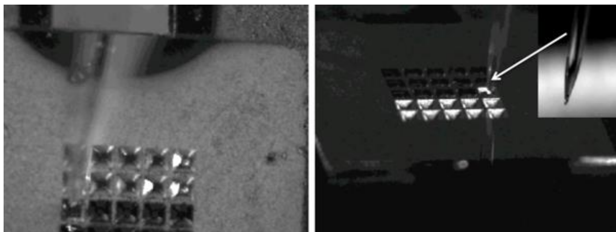
Figure S4 Microfabricated chip on the dew point stage as the nano-wells are filled with protein (crystallization) solution, with nanoliter accuracy. Left – top view; right – side view. The 5 x 5 well array is 2 mm x 2 mm in size. The automatic method was used to load each well with 15 nl of liquid. It took about 2 min. to load all 25 wells. See the Supplementary Movie for a demonstration.
