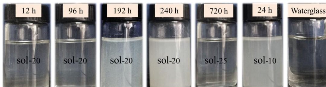
Figure S1 Appearance condition of aluminosilicate sols and water glass during the aging process for each period.
