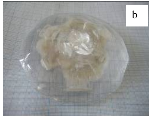
Fig. S4. Photographs of \beta -BaB 2 O 4 crystals grown in the 0.7 BaB 2 O 4 -0.3 LiBaF 3 system in the first growth cycle (a) and in the second growth cycle (b).
