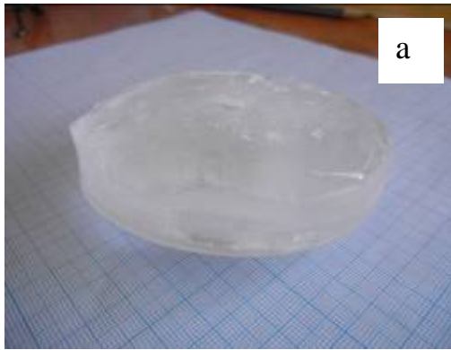
Fig. S4. Photographs of \beta -BaB 2 O 4 crystals grown in the 0.7 BaB 2 O 4 -0.3 LiBaF 3 system in the first growth cycle (a) and in the second growth cycle (b).
