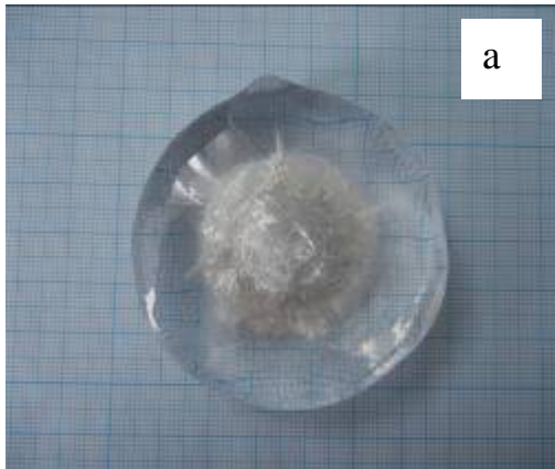
Fig. S4. Photographs of \beta -BaB 2 O 4 crystals grown in the 0.7 BaB 2 O 4 -0.3 LiBaF 3 system in the first growth cycle (a) and in the second growth cycle (b).
