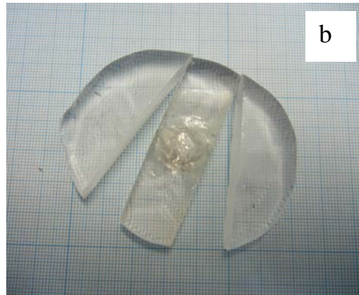
Fig. S4. Photographs of \beta -BaB 2 O 4 crystals grown in the 0.7 BaB 2 O 4 -0.3 LiBaF 3 system in the first growth cycle (a) and in the second growth cycle (b).
