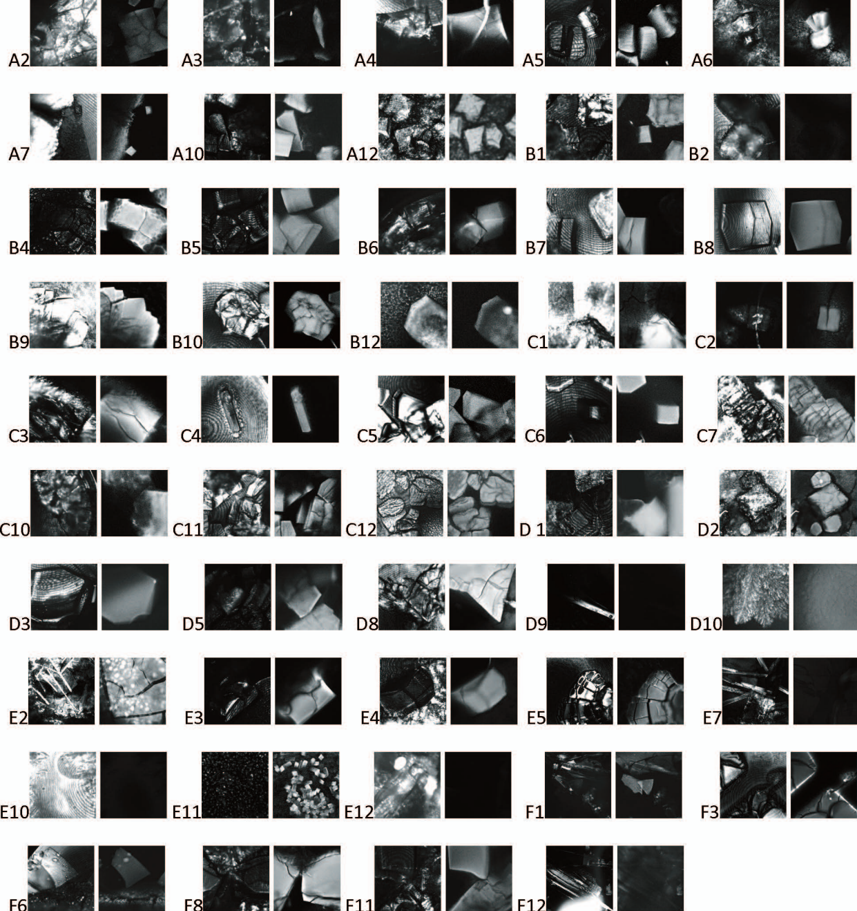
Figure S2 Pairs of confocal images from a screening tray obtained with the Zeiss LSM510 microscope using 488 nm excitation wavelength; left – reflective confocal, right – fluorescence confocal. Fluorescence is observed only from protein crystals, but not from salts or crystallized PEGs. List of imaged crystallization conditions can be found in Table S1.
