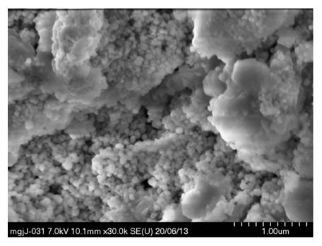
Zirconia nano-particles from SEM images were found to be on the order of 80-100nm in size, supported by structural refinement of pre laser-exposure powder diffraction patterns.
