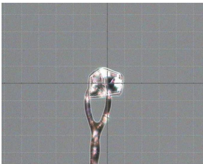
Figure S12 The small crystal used for measuring (III). One square grid is 0.1 x 0.1 mm.
