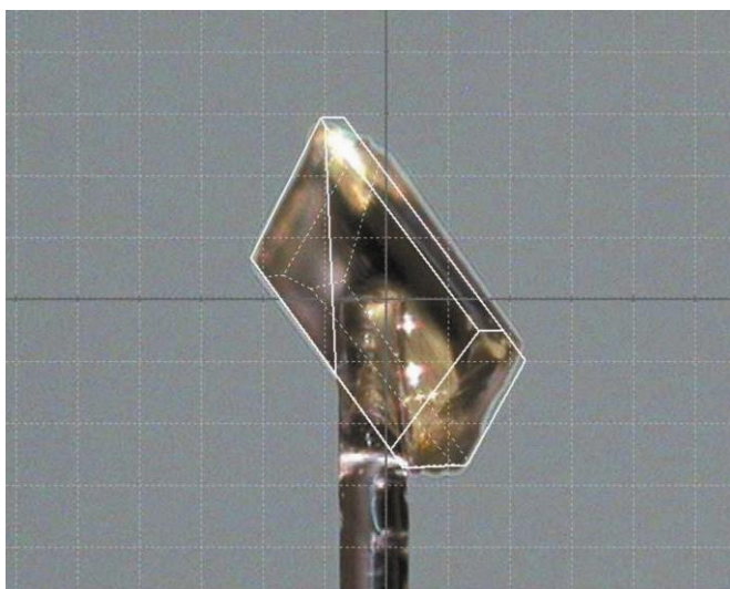
Figure S6 The large crystal used for measuring (II). One square grid is 0.1 x 0.1 mm.
