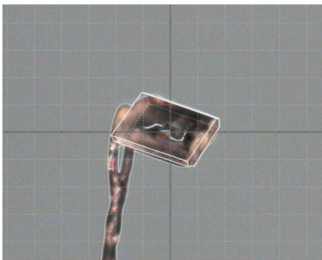
Figure S18 The large crystal used for measuring (V). One square grid is 0.1 x 0.1 mm.
