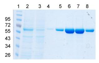
**Figure S2** SDS-PAGE image showing several steps of SGSH purification. Lane 1: Protein size markers, molecular weights are indicated at the left side in kDa. Lane 2: crude supernatant from cell culture containing recombinantly expressed SGSH. Lane 3: Flow through. Lane 4 and 5: Fractions eluted from the column at 100 mM imidazole. Lane 6 to 8: Fractions eluted from the column at 250 mM imidazole that were used for crystallisation trials.
