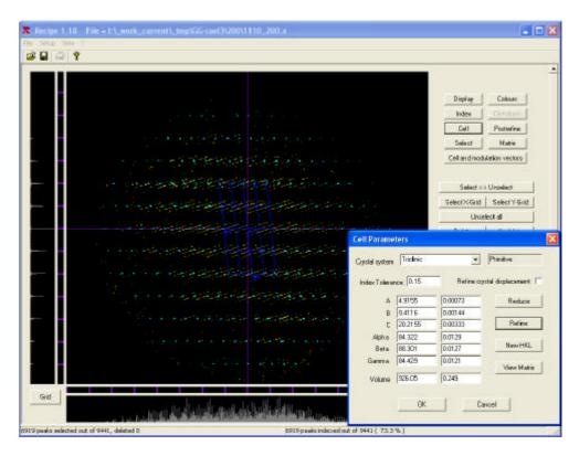
3) At this step we removed all indexed peaks from the reciprocal space view and projected all difference vectors for remaining peaks on the horizontal plane again with selection of 3 independent lines as described for the first step.
