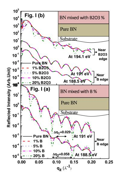
Figure I (For supporting material). Simulated SXRR profiles at selected photon energies near different absorption edges for an ideal (zero roughness) bilayer structure (Mixed BN (11 nm)-on-Pure BN (11 nm)) on Si substrate. The top mixed layer is uniformly mixed with different atomic percentages. (a) Mixing with different B at. % near B edge (b) Mixing with different  $B_2O_3$  at. % near B and  $B_2O_3$  edge.
