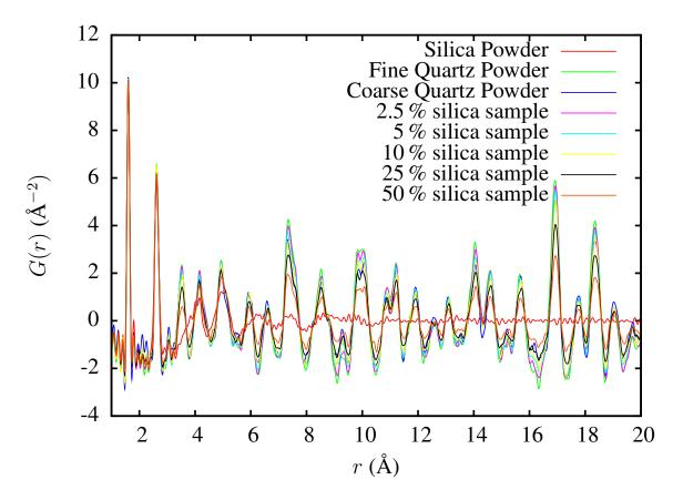
Fig. S2. Low-r region of the PDFs for the mixed samples, fine quartz, coarse quartz, and silica powder used in this study.
