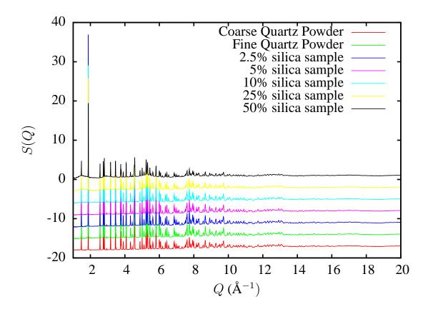
Fig. S1. Normalized total scattering pattern, S(Q), for the mixed samples, fine quartz, and coarse quartz powder. An offset has been applied for clarity.
