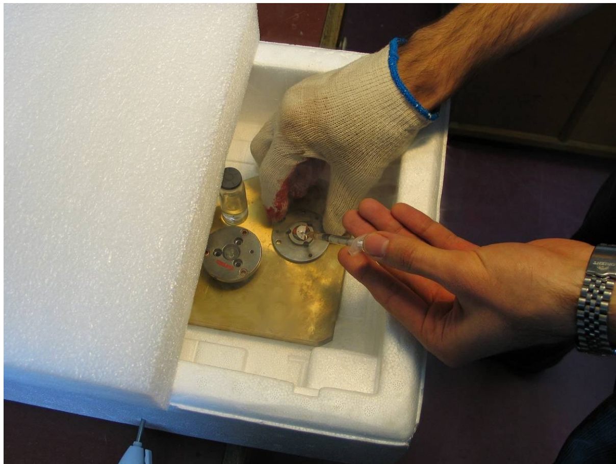
Figure B. Placing pentane:isopentane mixture (1:1) into gasket hole.
