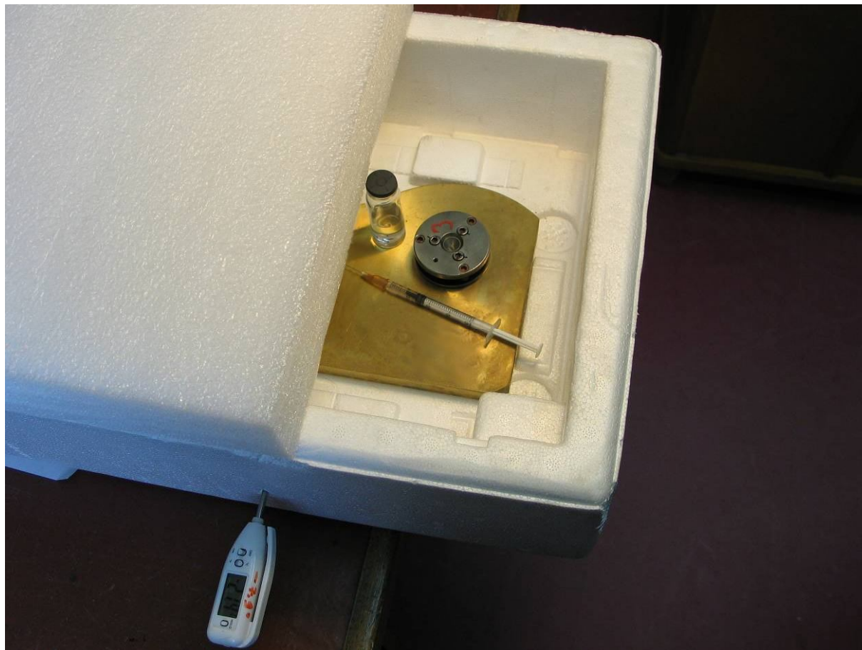
Figure A. Chamber prepared to the diamond anvil cell loading by pentane:isopentane mixture (1:1).
