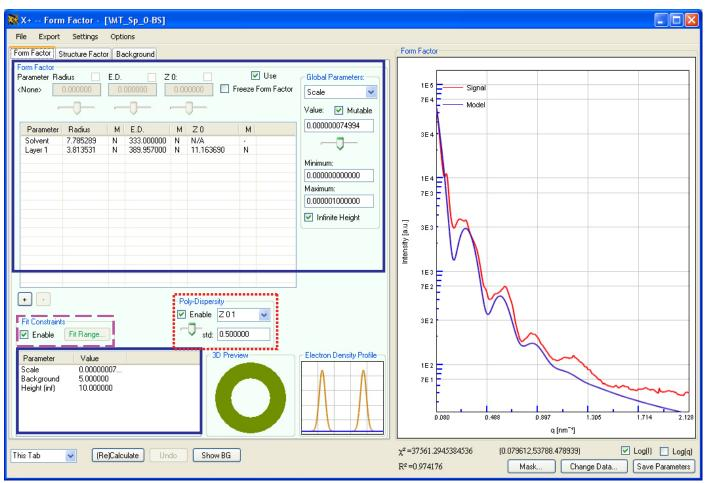
The Form Factor pane. The model's parameters are entered in the areas surrounded by the blue boxes. Polydispersity of a parameter is controlled in the red dotted box. Constraints and linked parameters are defined in the area surrounded by the dashed pink box.
