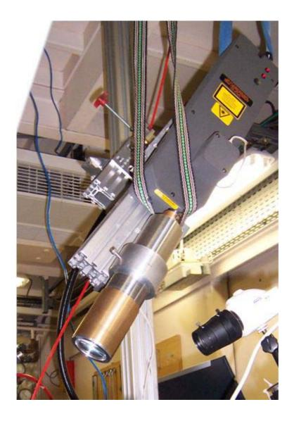
**Figure S2**: The Raman probe (RP in figure S1) equipped with the long distance optical expander (the optical head) allowing a long (150 mm) working distance.
