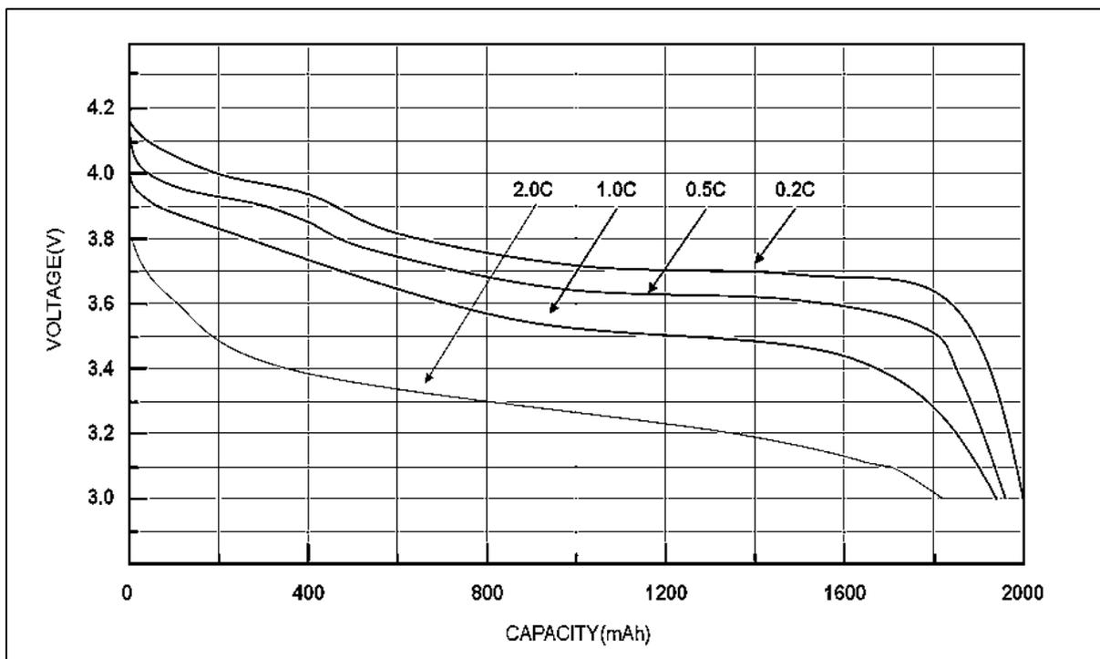
Figure 7 – Voltage vs. Drained Capacity During Discharging
