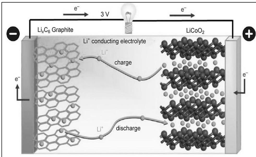
Figure 4 – Flow of Electrons During Discharging
