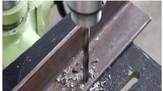
Fig: 5. Drilling of a L-Section
