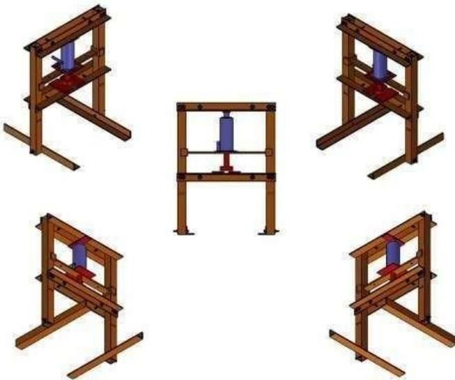
Fig: 11. Isometric view Of Hydraulic Press Machine
