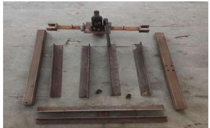
Fig: 6. Parts of Hydraulic Press
