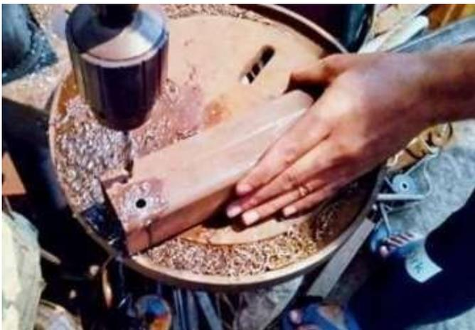
Fig: 4. Drilling of a Square Pipe
