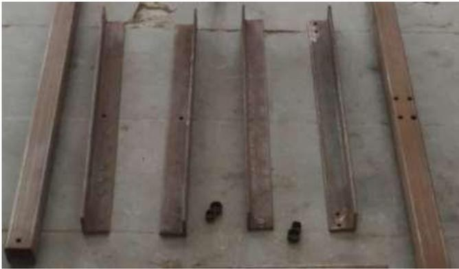
Fig: 3. L-Section and Square Pipe
