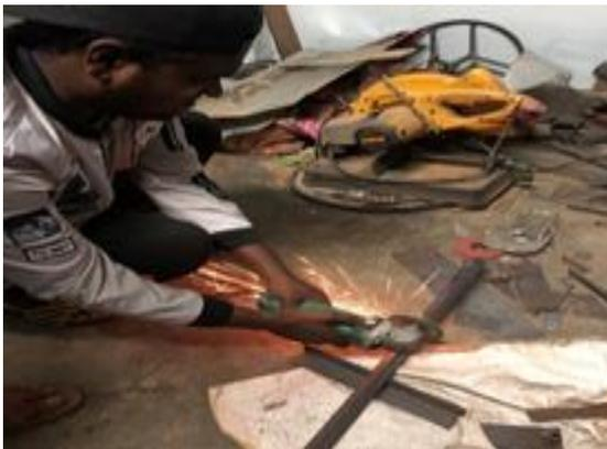
**Fig. 5.** Cutting of Supporting Rods
