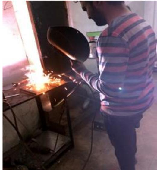
**Fig : 7.** Welding of Solar Panel Holder
