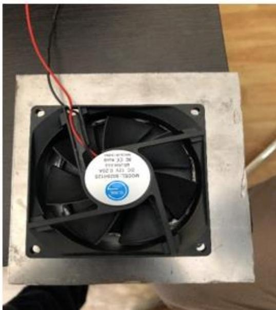
**Fig : 10.** Suction Fan Fixed to the Plate
