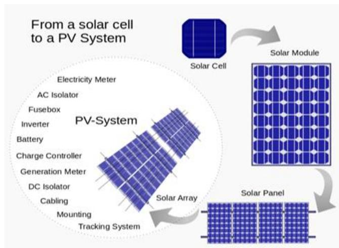
Fig : 1. From Solar Cell to a PV Cell
