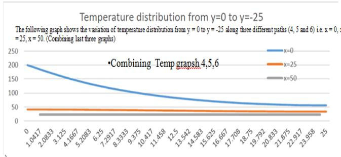
The following graph shows the variation of temperature distribution from y = 0 to y = -25 along three different paths (4, 5 and 6) i.e. x = 0, x = 25, x = 50. (Combining last three graphs)
