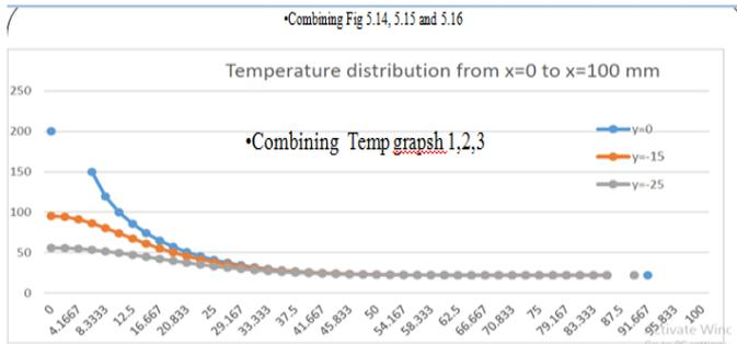
The following graphs shows the variation of temperature distribution from x = 0 to x = 100 along three different paths (1, 2 and 3) i.e. y = 0, y = -15, y = -25. (Combining first three graphs)
