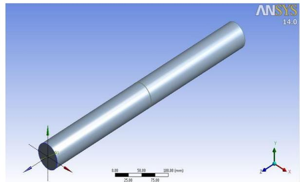
In this analysis we assume a uniform heat source of temperature 5000°C acting along a width of 10 mm along the surface of the workpiece. In the above figure a small circle can be seen (from z=245 mm to z= 255 mm) which is the heat affected region.
