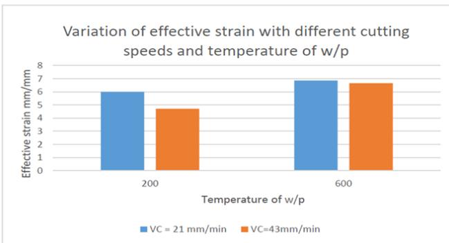
It can be seen that the effective strain decreases with increase in cutting speed, other parameters remaining same. But for a given cutting speed the effective strain increases with increase in temperature of work piece
