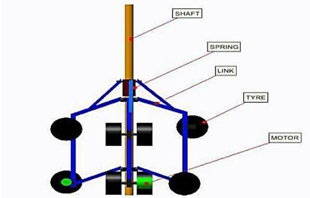
Figure 3. Duct Cleaning Set up
