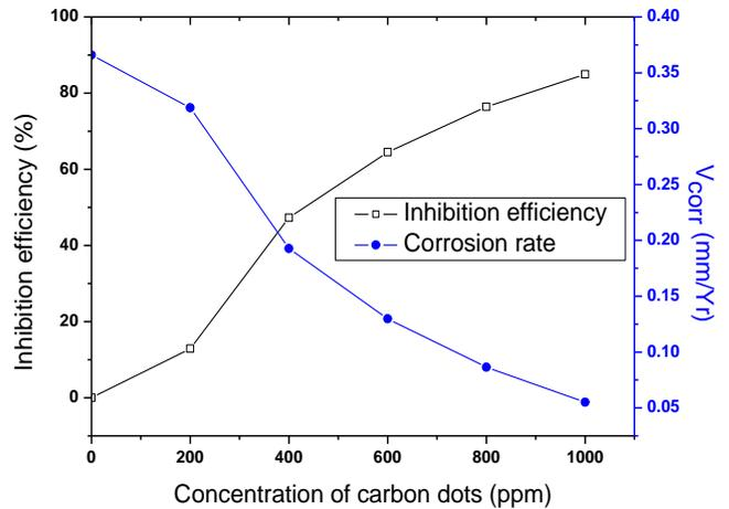
**Figure 8.** The corrosion rates and inhibition efficiencies for copper in different concentrations of coffee carbon dots in 1% NaCl solution.
