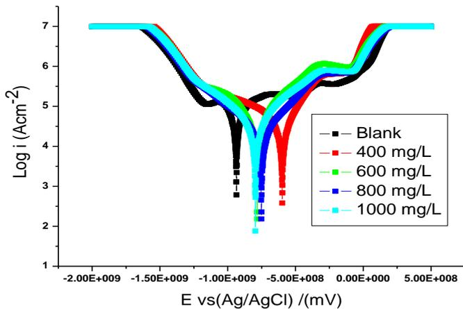
**Figure 9.** The Tafel polarization curves of copper in 1% NaCl at different carbon dot concentrations.
