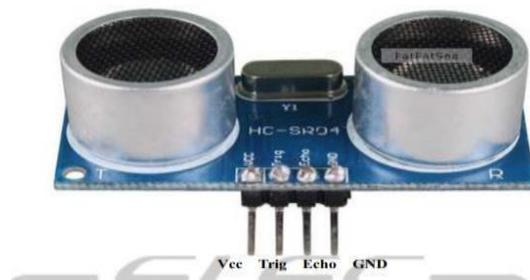
Ultrasonic device module consists of four pins:
