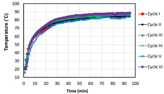
Fig. 6. Heating temperature history of the bed ( $100^{\circ}\text{C} - 20^{\circ}\text{C}$ )
