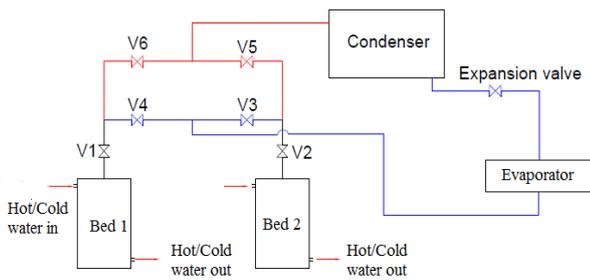
Fig. 2. Schematic of Adsorption System
