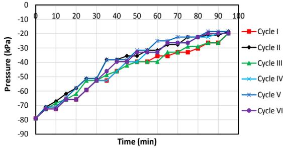
**Fig. 8. Heating pressure history of the bed (100°C - 20°C)**
