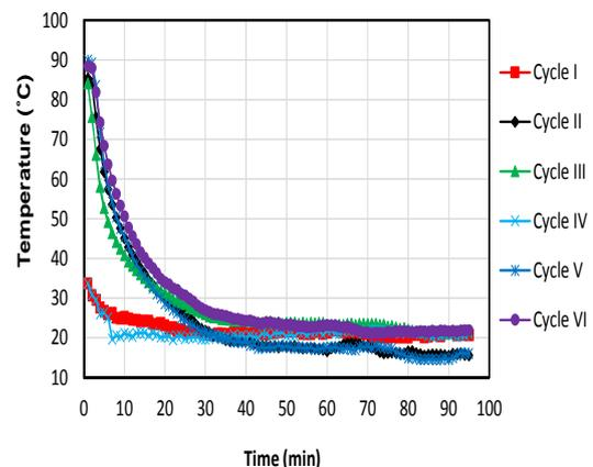
Fig. 7. Cooling temperature history of the bed ( $100^{\circ}\text{C} - 20^{\circ}\text{C}$ )
