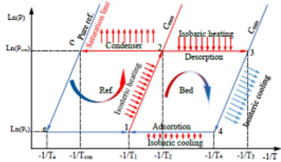
Fig. 3. Clapeyron Diagram for Adsorption Cycle
