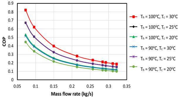
Fig. 13. Effect of Hot Water Flow Rate on COP
