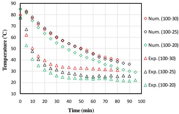
Fig. 12. Temperature of Bed by Using  $T_{h, w} = 100^{\circ}\text{C}$
