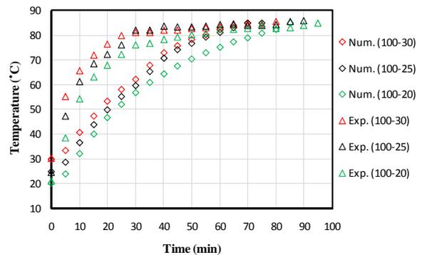
**Fig. 11. Temperature of Bed by Using  $T_{h,w} = 100^\circ\text{C}$**
