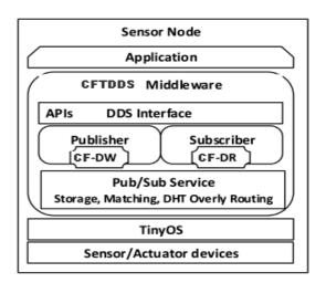
Figure 1: CFTDDS Architecture
