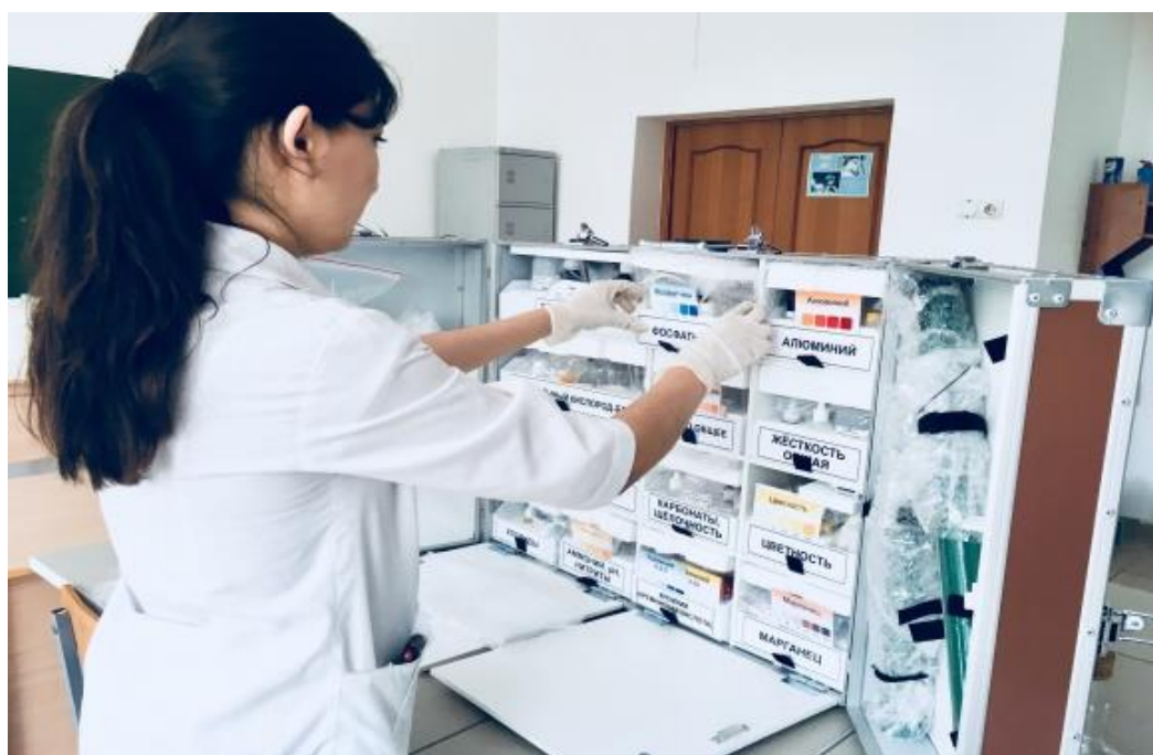
Figure 1. The study of the hydrochemical regime of water was carried out using the NKV-12 Express laboratory
