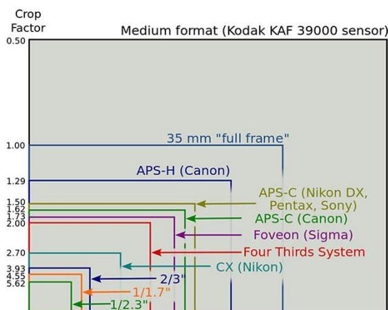
Figure 1. Image sensor size comparison
