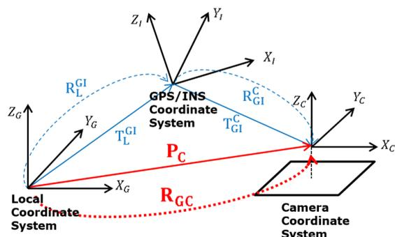
Figure 8. Coordinate systems and involved parameters in the system calibration
