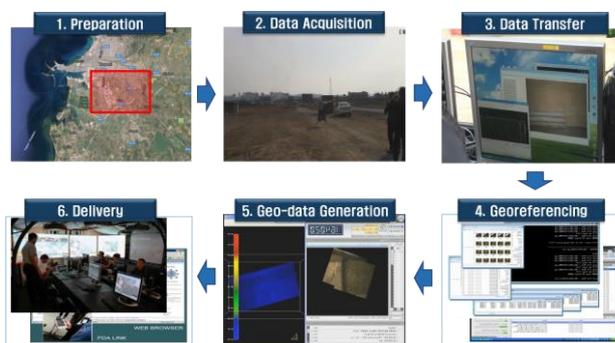
Figure 2. Operation concept of the UAV mapping system
