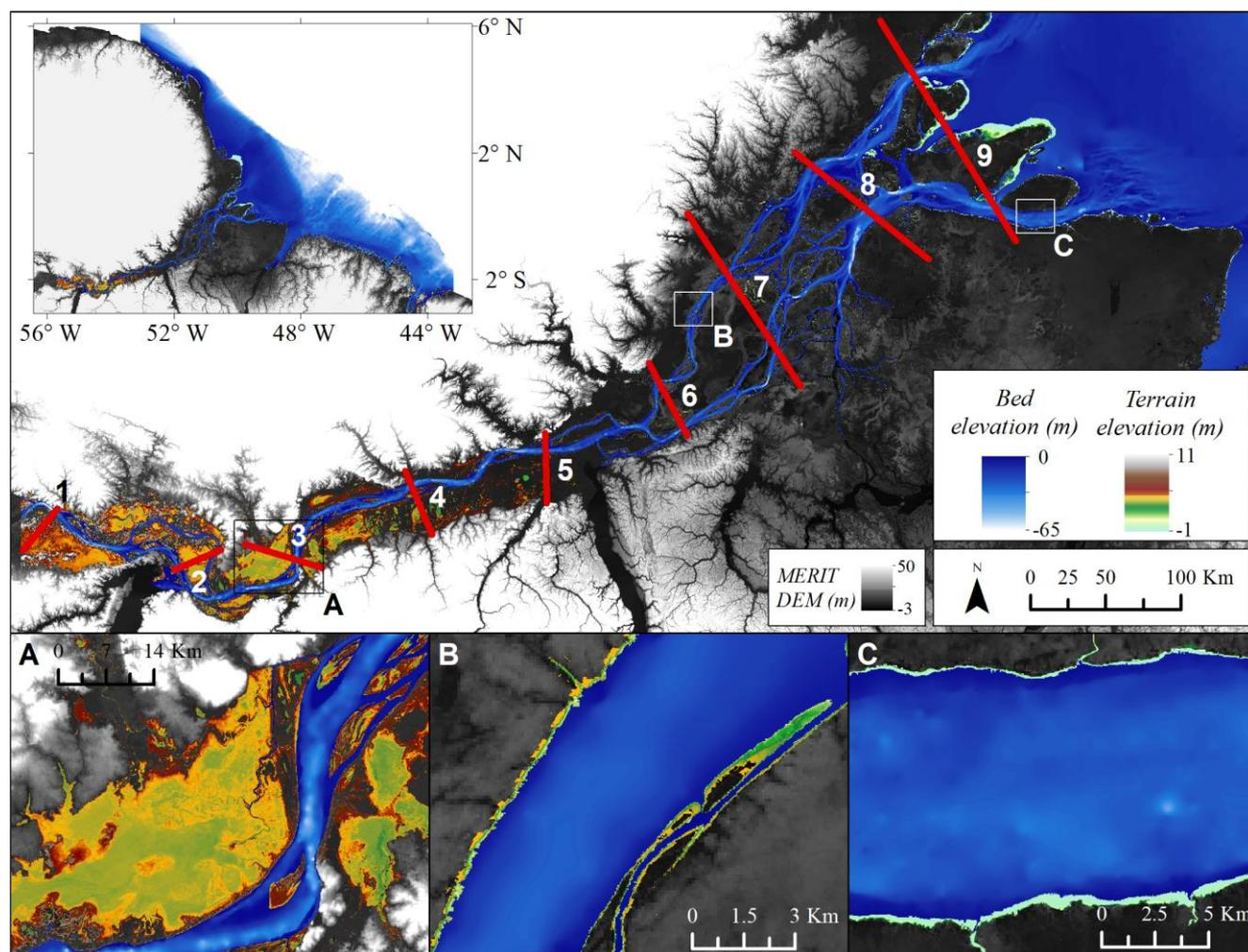
Figure 6. Estimated topography and bathymetry of the Amazon estuary with MERIT DEM and GEBCO 2020 data.
