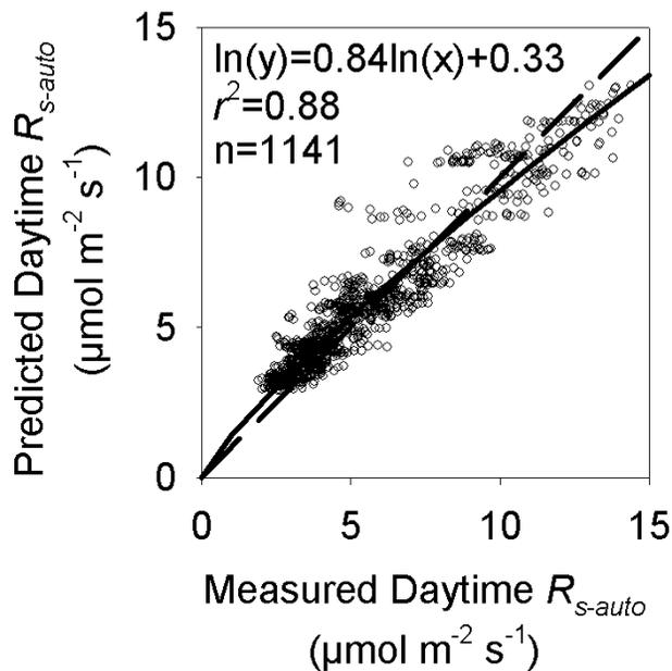
**Fig. 1.** Relationship between predicted (with the gap-filling algorithm) and measured daytime soil respiration ( $R_s$ ) for three periods in 2004 when chambers were darkened (18–19 July , 27 August – 1 September and 22–24 September). A log transformation was used on both x and y to provide homoscedasticity. Given the error associated with x, a geometric mean regression was used.
