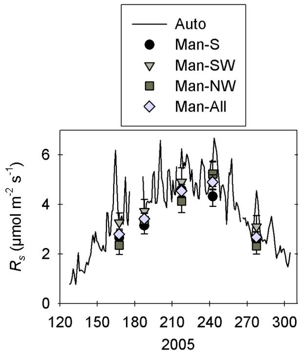
**Fig. 2.** Time series of automated (Auto; daily mean of non-gap-filled nighttime measurements) and manual (Man) soil respiration ( $R_s$ ) measurements for three sectors of the tower footprint.
