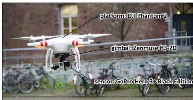
Figure 2: Platform and sensor used in this study
