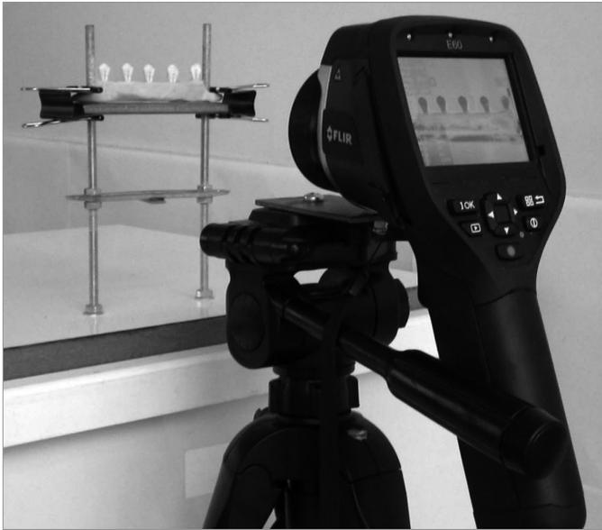
Figure 1. Thermal imaging of sample teeth from a 15 cm distance
