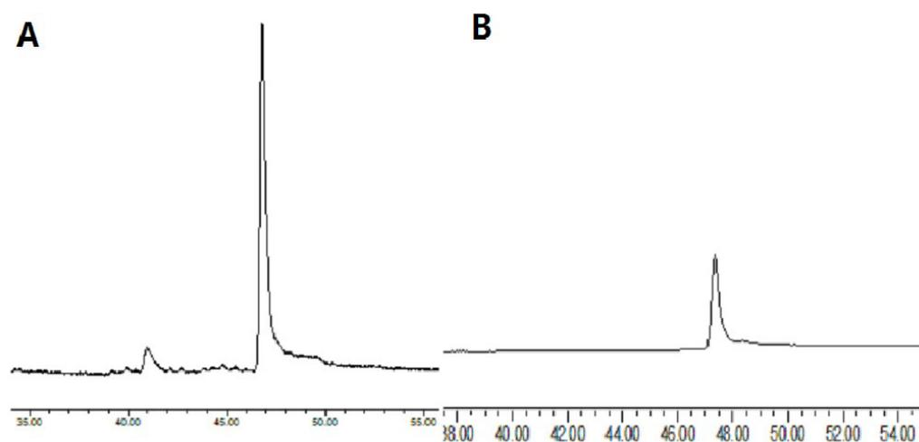
**Figure 3.** HPLC analysis of the reaction products catalyzed by purified recombinant MrFPS incubated with GPP and IPP. **A.** Standard (FPP) chromatogram. **B.** Sample (purified recombinant MrFPS incubated with GPP and IPP) chromatogram.
