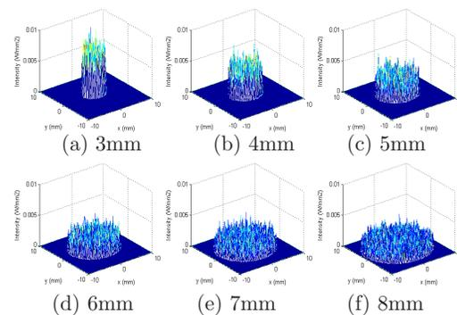
Fig. 3. Intensity distributions of emergent light (the incident rays with 5° field of view, the pupil diameters of: (a) 3, (b) 4, (c) 5, (d) 6, (e) 7, and (f) 8 mm).
