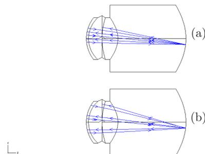
Fig. 1. Schematic plots of optical model of bright pupil effect at the pupil diameters of: (a) 3 and (b) 6 mm.
