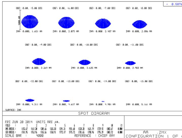
Fig. 2. Spot diagram of emergent light (incident rays with 5°–15° field of view).
