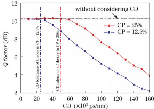
Fig. 5.  $Q$  factor versus CD with  $N_{TS}=6$  and  $OSNR=13$  dB.
