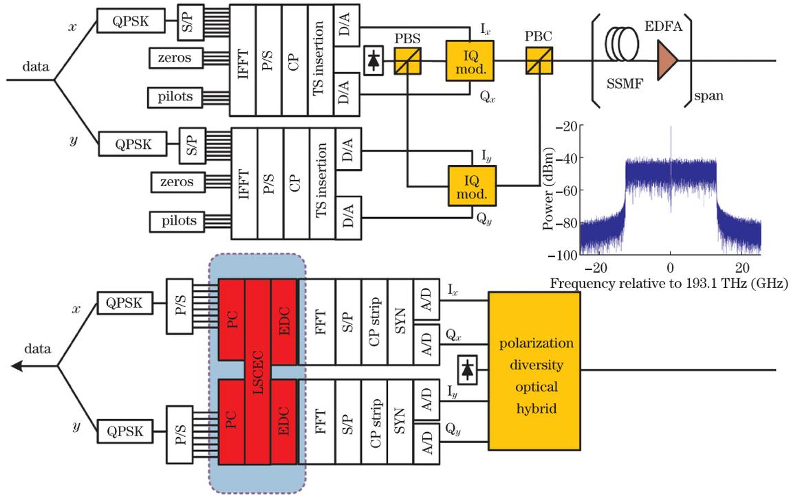
Fig. 1. Setup of 100-Gb/s PDM-CO-OFDM system. S/P: serial-to-parallel.
