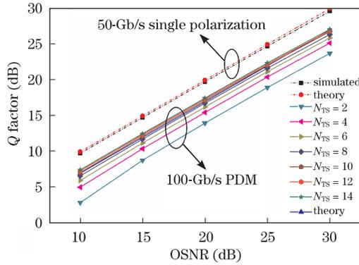
Fig. 3.  $Q$  factor versus OSNR in B2B.
