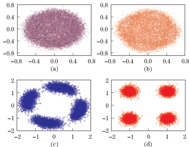
Fig. 9. Constellations for the compensator in receiver after 800 km with input power in the first span equal to  $-2$  dBm (a) before EC; (b) after EDC in EC; (c) after LSCEC in EC; (d) after PC in EC.
