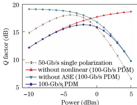
Fig. 8.  $Q$  factor versus input power into the first fiber span for different circumstances after 800 km.
