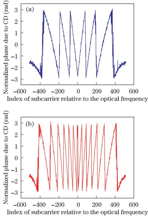
Fig. 4. Phases of the subcarriers estimated by EDC with  $N_{TS}=6$ ,  $CP=25\%$  and  $OSNR=13$  dB for (a) 5000 and (b) 10000 ps/nm.
