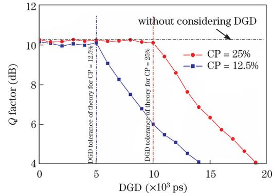
Fig. 6.  $Q$  factor versus DGD with  $N_{TS}=6$  and  $OSNR=13$  dB.
