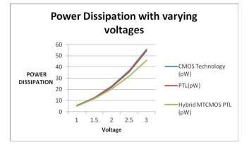
Fig 8 Average power dissipation of 2:1 MUX using CMOS Technology, PTL and Hybrid MTCMOS PTL at different voltages
