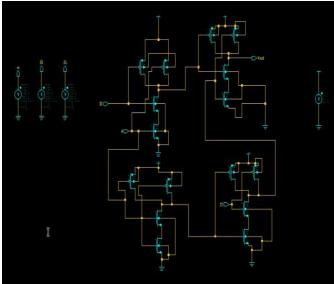
Fig 2 MUX using CMOS Technology
