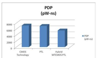
Fig 9 Power Delay Product (PDP) of 2:1 MUX at 3.3V
