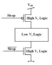
Fig 1 power gated circuit
