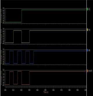
Fig 6 Simulation result of MUX using PTL
