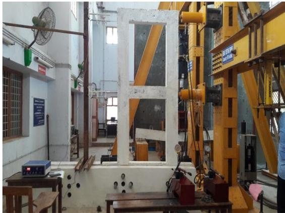
**Fig.3 Testing of RC Frame Model**
