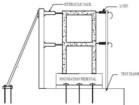
**Fig.2 Test Setup of RC Frame Model**
