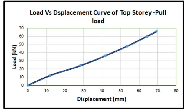
Fig.10 Load Vs Displacement curve for RC frame for Top storey – Pull type loading
