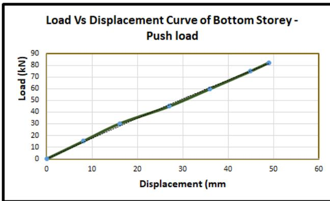
Fig.7 Load Vs Displacement curve for RC frame for bottom storey – Push type loading
