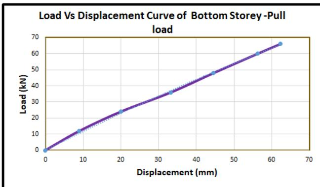
Fig.8 Load Vs Displacement curve for RC frame for bottom storey – Pull type loading
