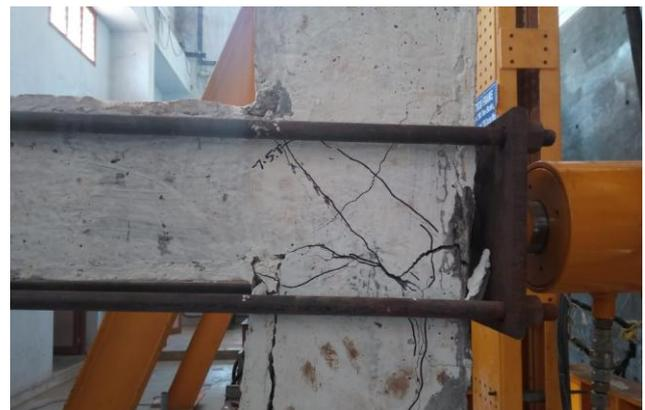
**Fig.6 Crack pattern at beam column joint at loading end**
