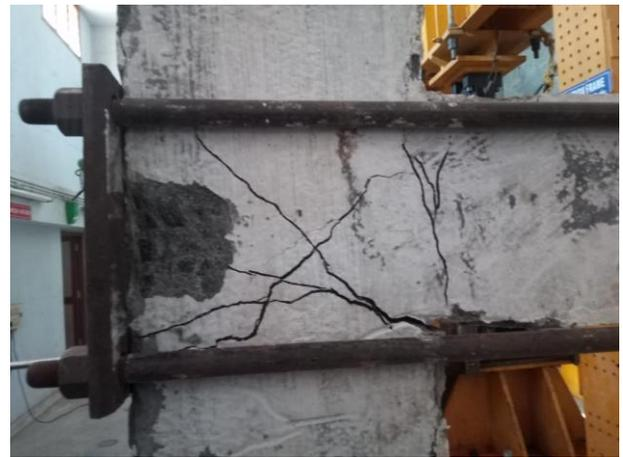
**Fig.5 Crack pattern at beam column joint at the opposite to loading end**
