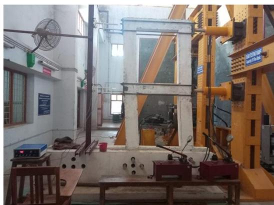
**Fig.4 Testing of RC Frame Model**
