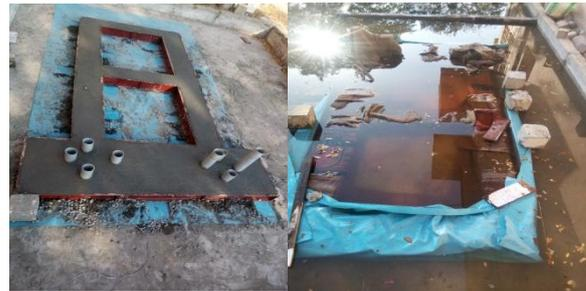
Fig.1 Casting and curing of RC frame model
