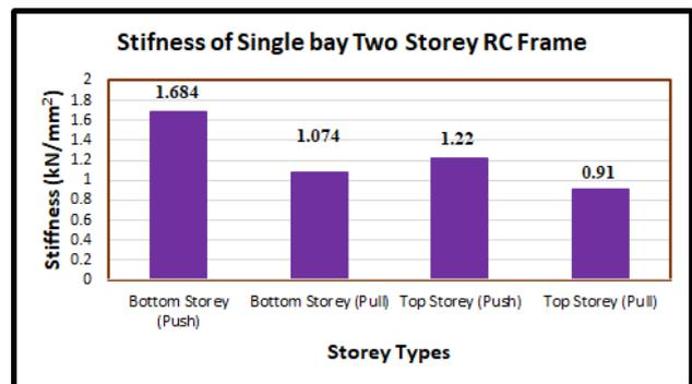
Fig.11 Stiffness characteristics of RC frame model
