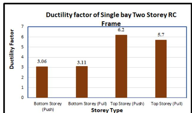
Fig.12 Ductility characteristics of RC frame model
