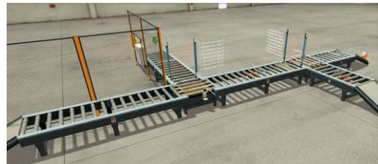
Fig. 5. Production line controlled by Siemens S7-1214DC controller, visualization done in Factory I/O
