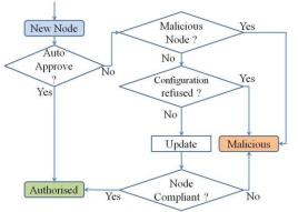
Fig. 4. Access Control in IoT
