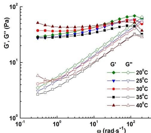
Figure 4: Variation of  $G'$  and  $G''$  moduli of C2 at five temperatures
