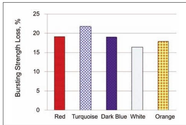
Fig. 5. Bursting Strength Results Before and After Sunlight Exposure (a); Bursting Strength Loss After Sunlight Exposure (b)
