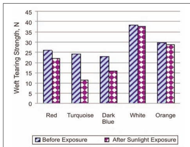
Fig. 6. Tearing strength test results
