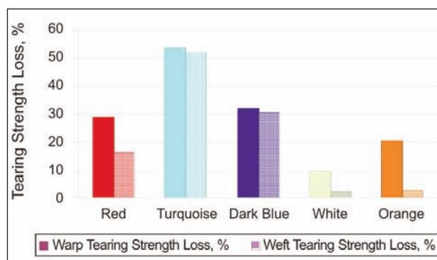
Fig. 7. Tearing strength loss after sunlight exposure
