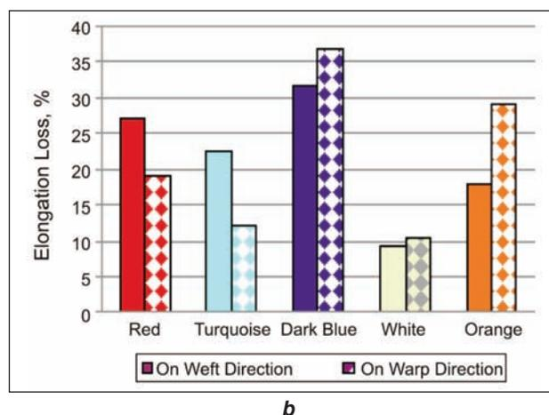
Fig. 4. Breaking Strength Loss and Elongation Loss of the Fabrics
