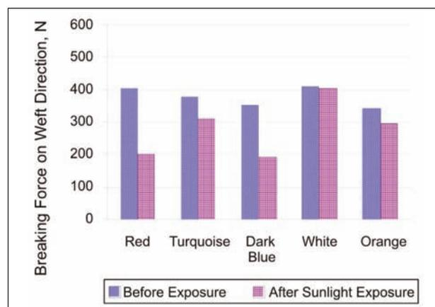
Fig. 2. Breaking Force Results: *a* – on Warp Direction; *b* – on Weft Direction
