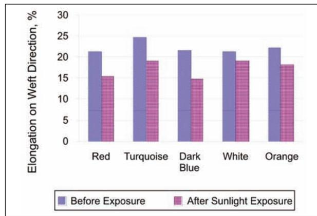
Fig. 3. Elongation Results: a – on the Warp Direction; b – on the Weft Direction
