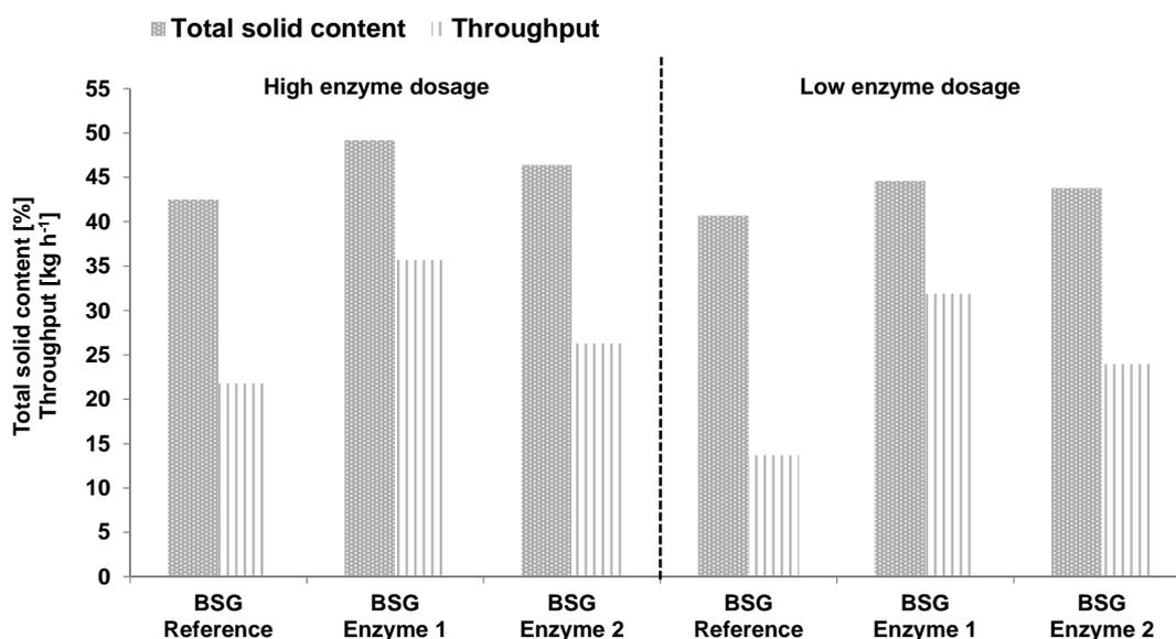
Figure 3: TS content and throughput of enzymatic and mechanical pre-treated BSG
